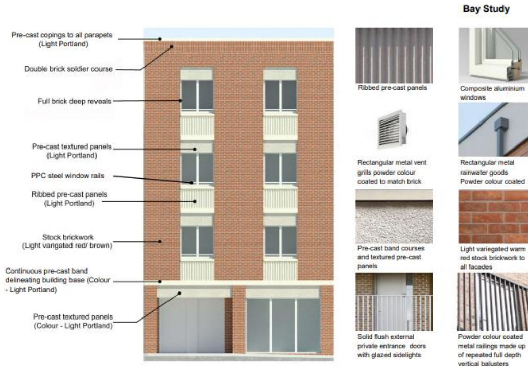
Figure 7: Materials and detailing
